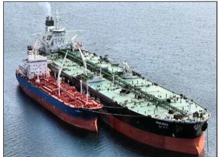
Example: Crude oil tanker performing STS with smaller product tanker
